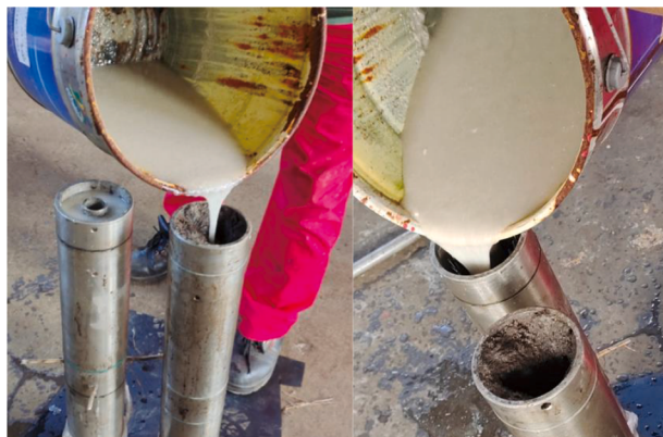
Fig. 16. Unheated state of gel plugging agent.
