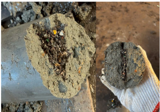
8 mm-coir fiber and vermiculite (e) 8 mm core section
