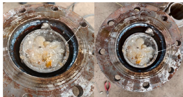
Fig. 17. Gel state after heating in water.
