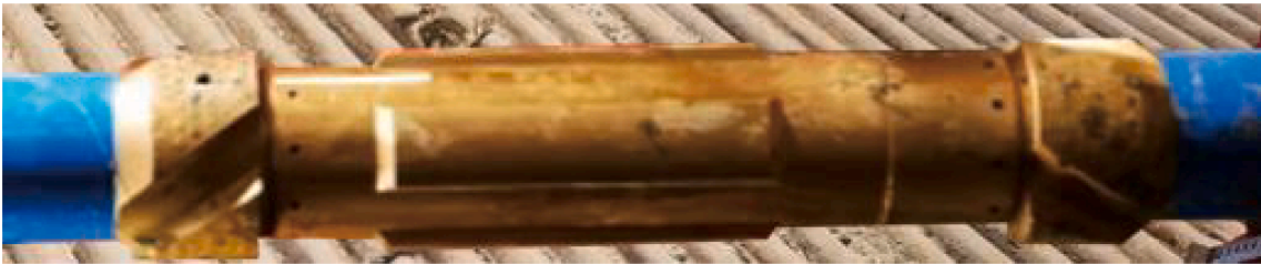
(c) VCRT external structure
