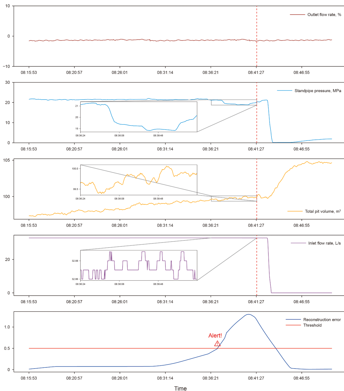
Fig. 14. Real-time logging data and kick risk warning results for Well 2 (the red dashed line represents the time when the field engineer issued the kick alarm).
