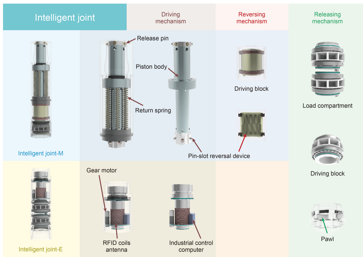
Fig. 15. Structural design of the intelligent joint.
