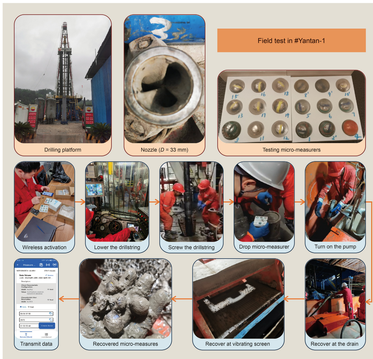
Fig. 10. Process of field test in #Yantan-1.
