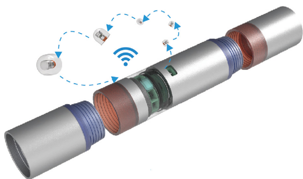
Fig. 16. Downhole IoT system based on micro-measurers and intelligent joint.
