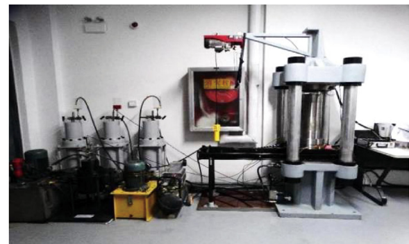
Fig. 3. Experimental apparatus for acid fracturing.
