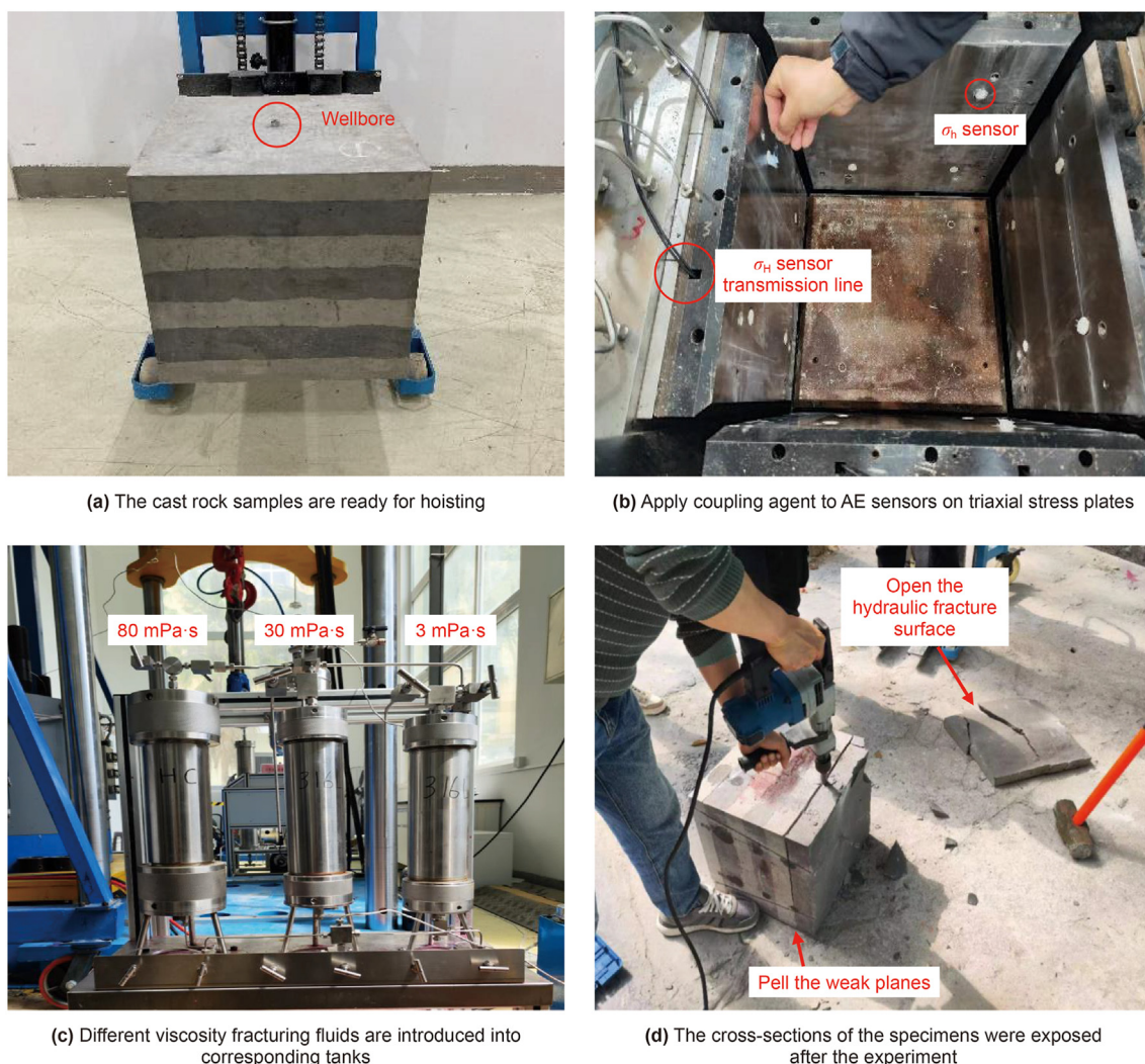
Fig. 3. Schematic diagram of the experimental process.
