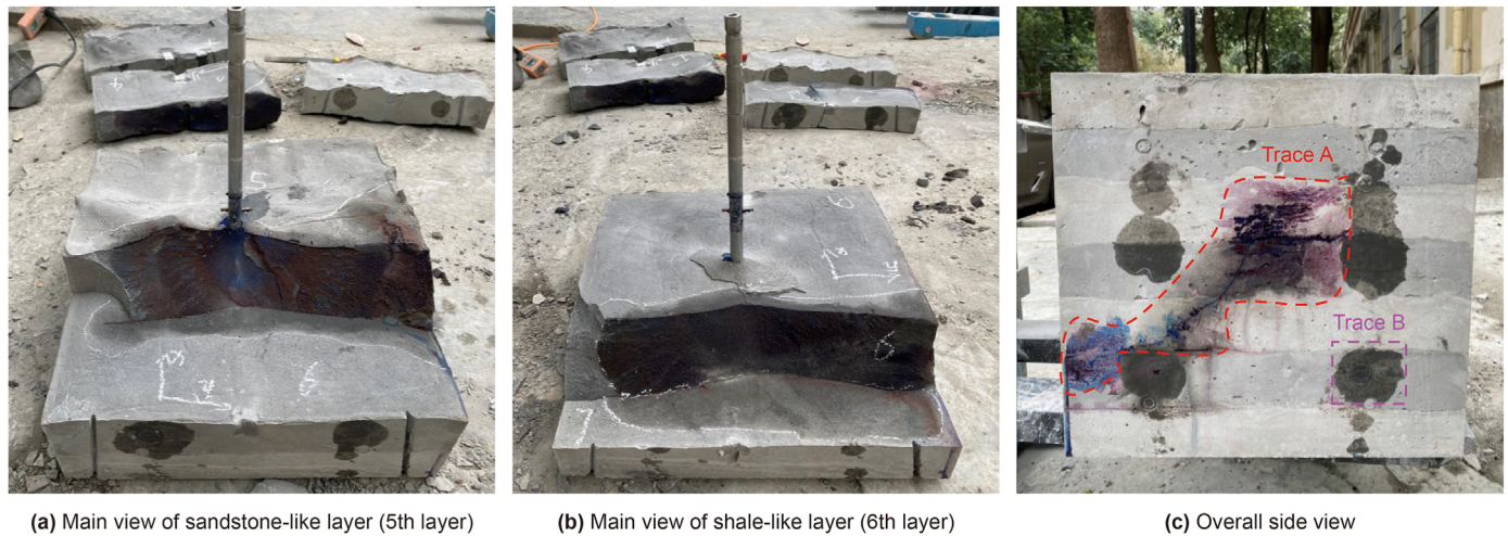
Fig. 5. Fracture morphology after the experiment for Sample #2.
