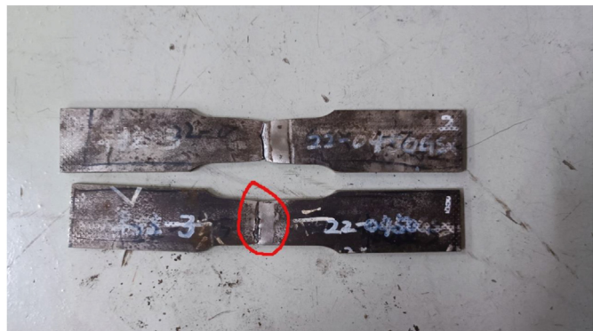
Fig. 9. Photo of girth weld tensile specimen.
