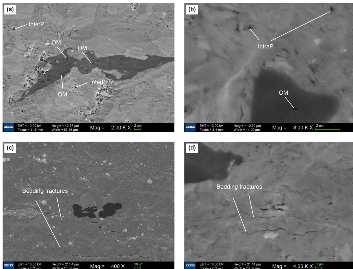
Fig. 4. Pore types in the shale samples observed by SEM images. (a) and (b) are view fields of the shale matrix; (c) and (d) are view fields of the shale bedding fractures.
