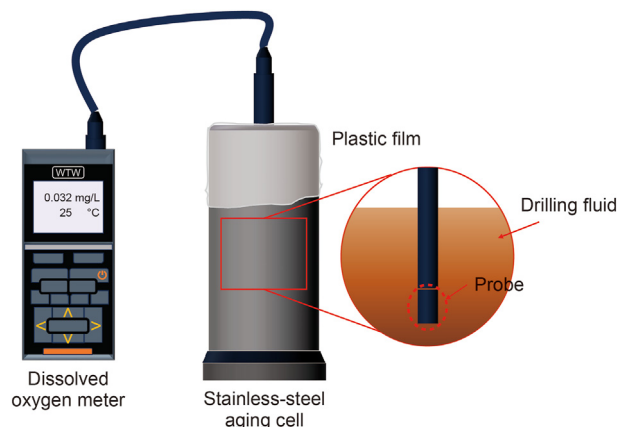
Fig. 2. Scheme of soluble oxygen concentration measurement.
