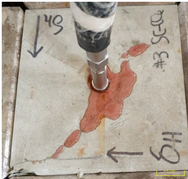
Fig. 8. Fracture obtained through dye fluid injection.
