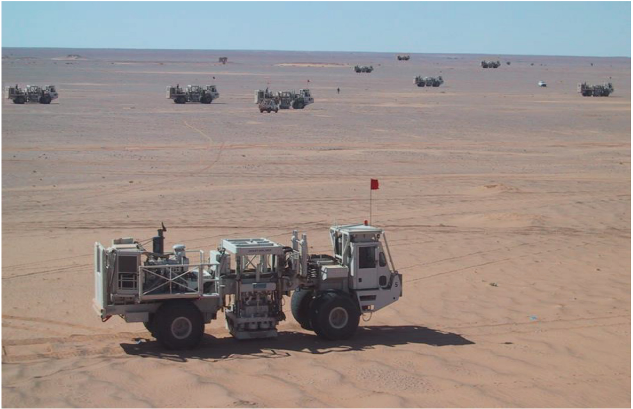
(a) A land vibroseis acquisition
