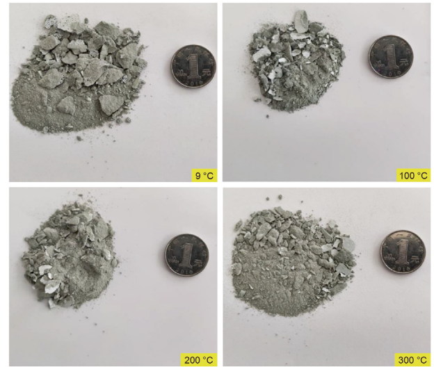
Fig. 20. The cutting chips of whole-cutter cutting.
