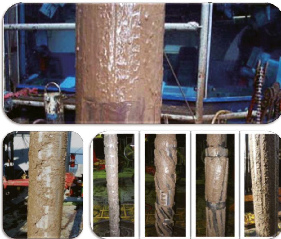
Fig. 1. Downhole drilling fluid contamination in the field.
