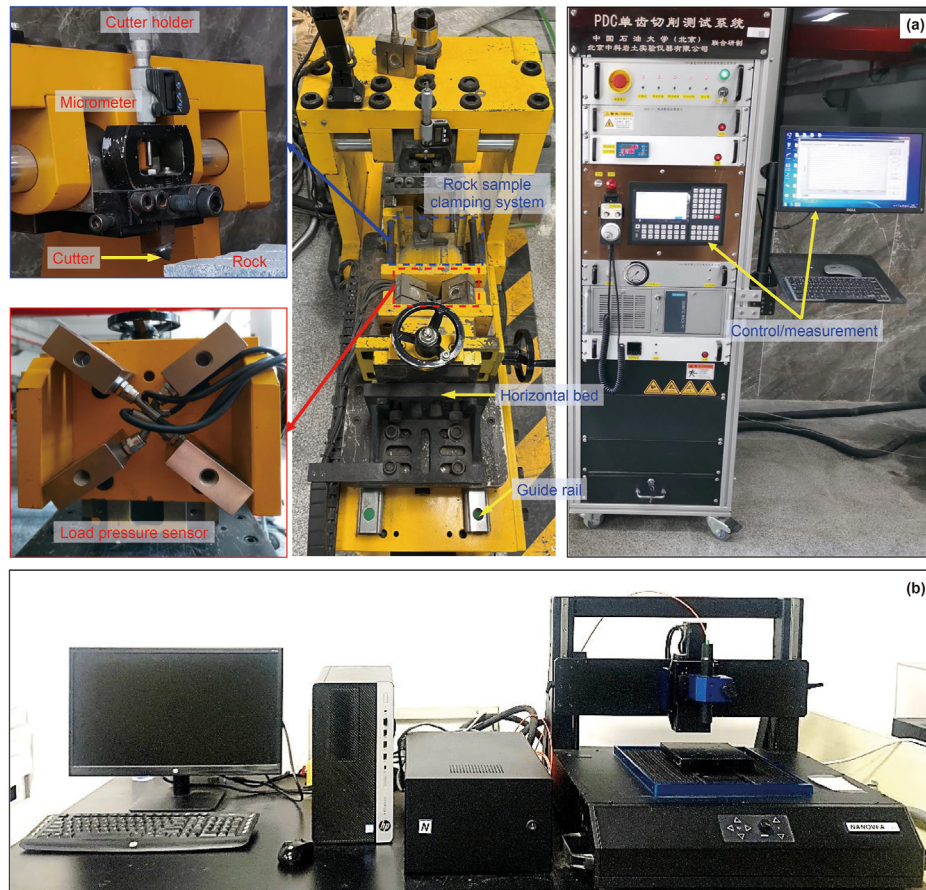
Fig. 2. Single cutter cutting and rock-breaking device (a); ST400 3D Profilometer (b).
