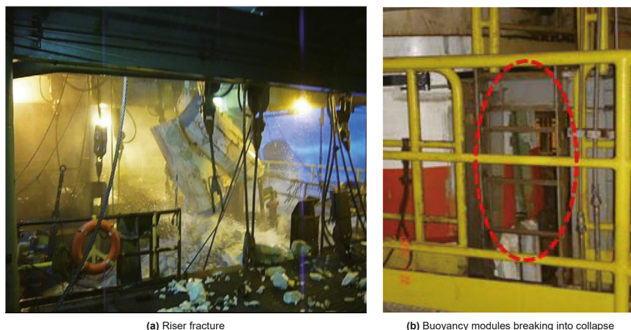
Fig. 1. Failure accidents of risers during typhoon conditions in the South China Sea.
