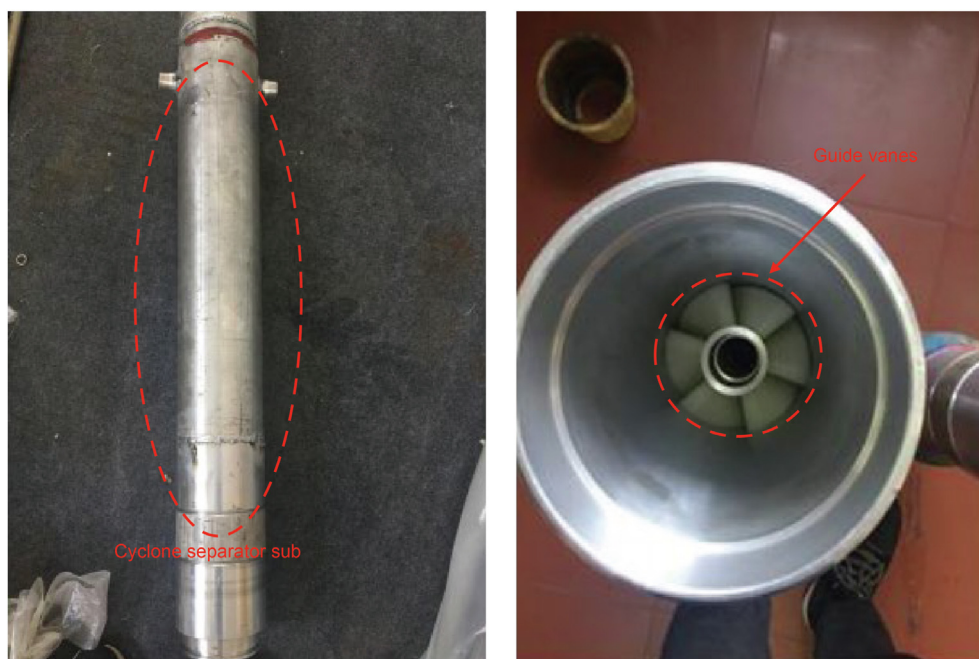
Fig. 2. The cyclone separator sub and guide vanes.
