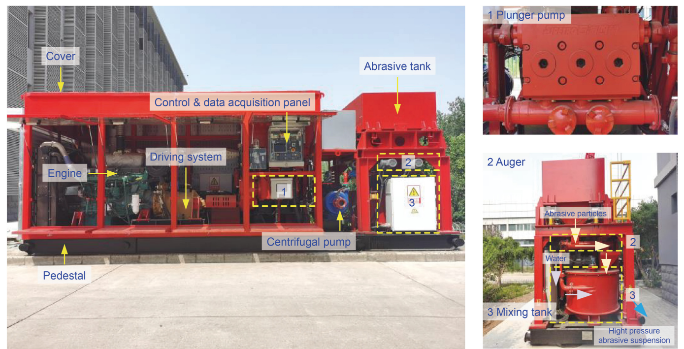
Fig. 4. Physical map of the high-pressure abrasive waterjet rock breaking laboratory system.
