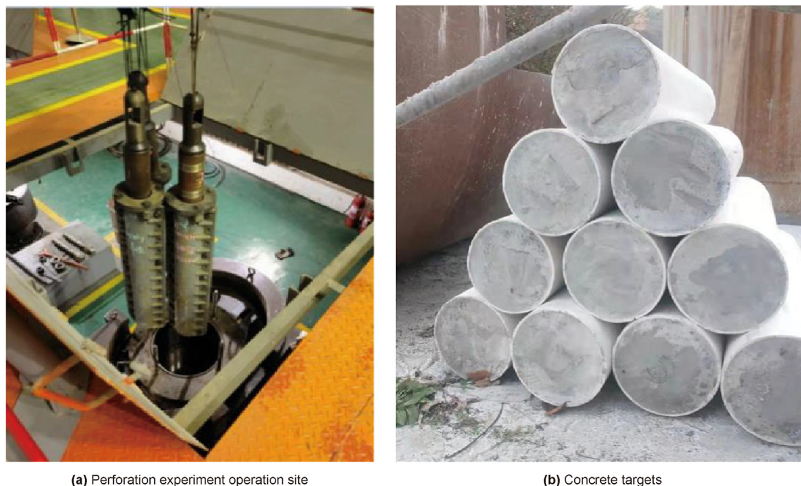
Fig. 8. High temperature and high-pressure perforating charge perforation experiment process.
