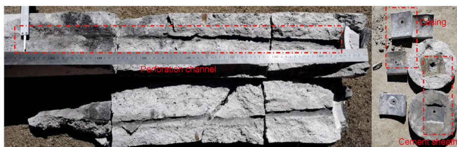
Fig. 9. Concrete target and casing after the high temperature and pressure experiment.
