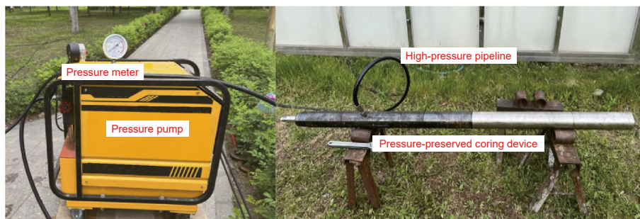
Fig. 28. Pressure-bearing performance test of the pressure-preserved coring device.
