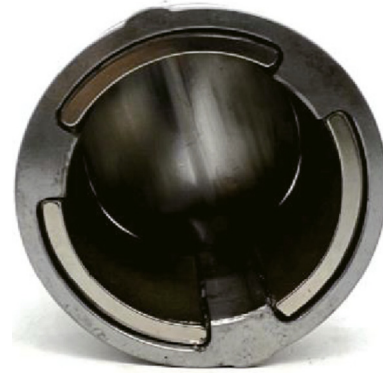
Fig. 18. Magnetically controlled self-sealing pressure-preserved controller.
