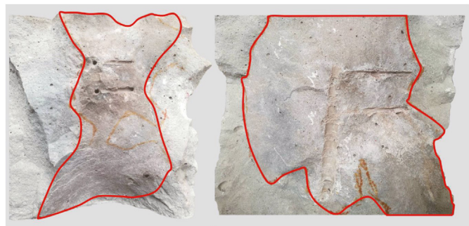
Fig. 6. The results of fracture recognition (the red curves represent fracture contours).
