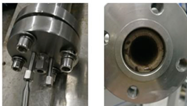
(b) 1D sandpack with temperature measuring function and thermal-insulating layer
