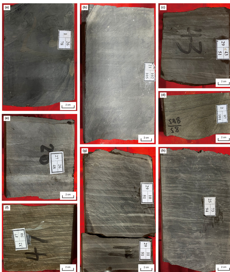
Fig. 6. Core photos showing the lithology and the three types of lamina structure of the Lucaogou Formation in the Jimusar Sag
