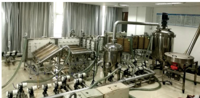
Fig. 14. Visual proppant sedimentation and transportation device.
