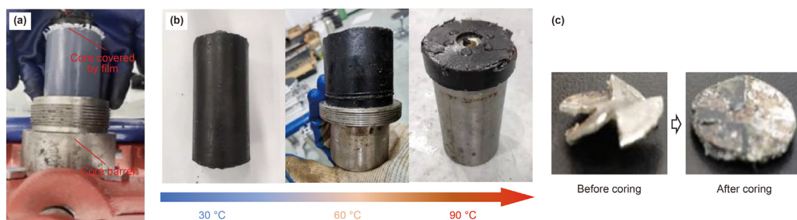
Fig. 7. a Demolding process of the film-forming core sample. b Film-forming core sample at 30°C, 60°C and 90°C. c In-situ impeller mixer units.
