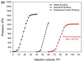
Fig. 9 Injecting pressure change of (a) HICDs and (b) HOCDs nanofluid with water flooding first, then the injection of HICDs or HOCDs nanofluid and subsequent water flooding
